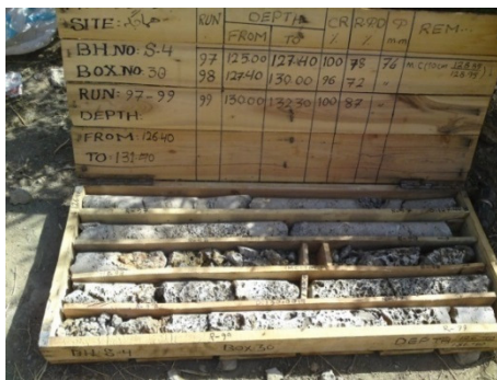
Fig. 2. S4 borehole in the Zimkan area from depths of 125-132 meters - porous rocks
