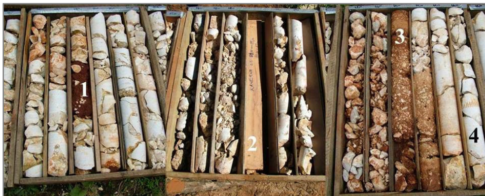
Fig. 3. Different materials in the rock mass of Zadar borehole: (1) terra rossa; (2) cavern; (3) rock fragments and terra rossa – partially solidified; (4) fractured rock.
