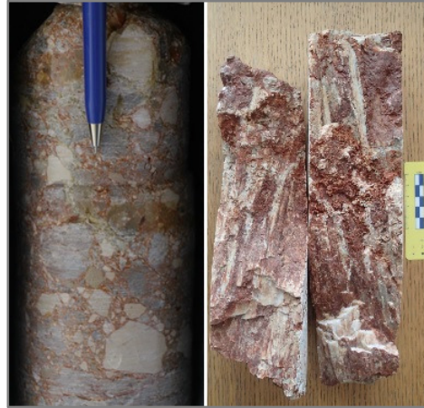
Fig. 4 Compact Jelar breccia (left) and a fracture with striations (right)
