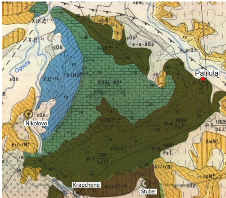
Fig. 2. Fragment of the geological map (Filipov, 1995a) (aQ – Quaternary gravel, sand, loess; N1s – Neogene clay, sand, limestone; sK1h-b – Salash Formation - limestone, marls)
