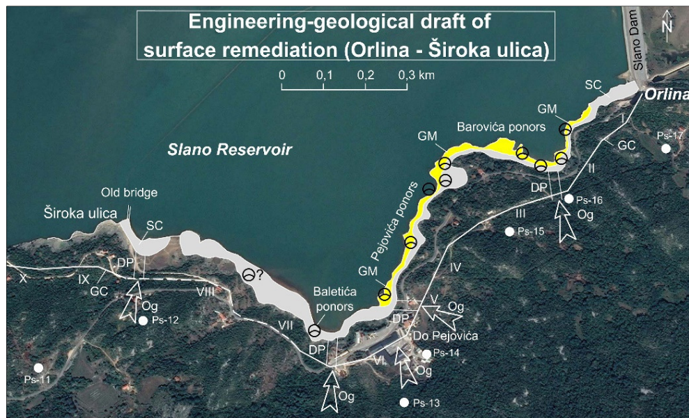
Fig. 3. Engineering-geological draft of the Slano Reservoir with a route for suggested waterproofing works. Legend: See Figures 2 and 4
