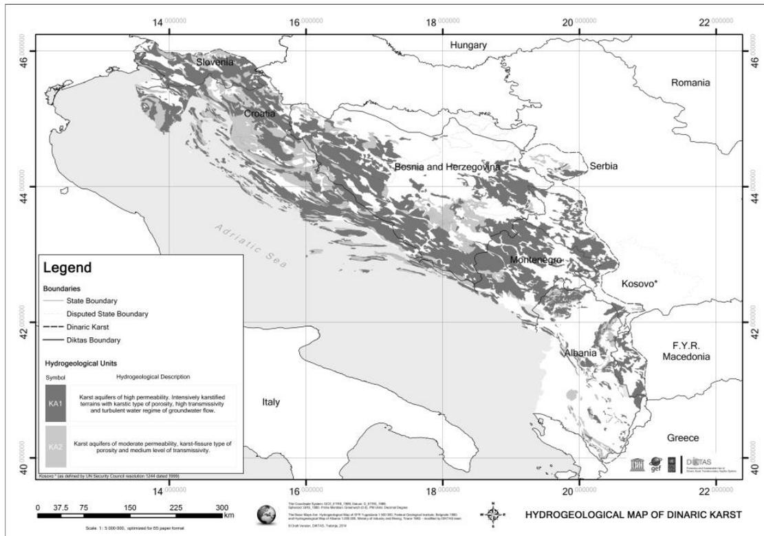
Fig. 1 Extension of Dinaric karst from Italy to Albania. The two types of karst aquifers are distinguished: KA1 – highly permeable and rich in groundwater reserves, and KA2 of moderate permeability and groundwater reserves.
